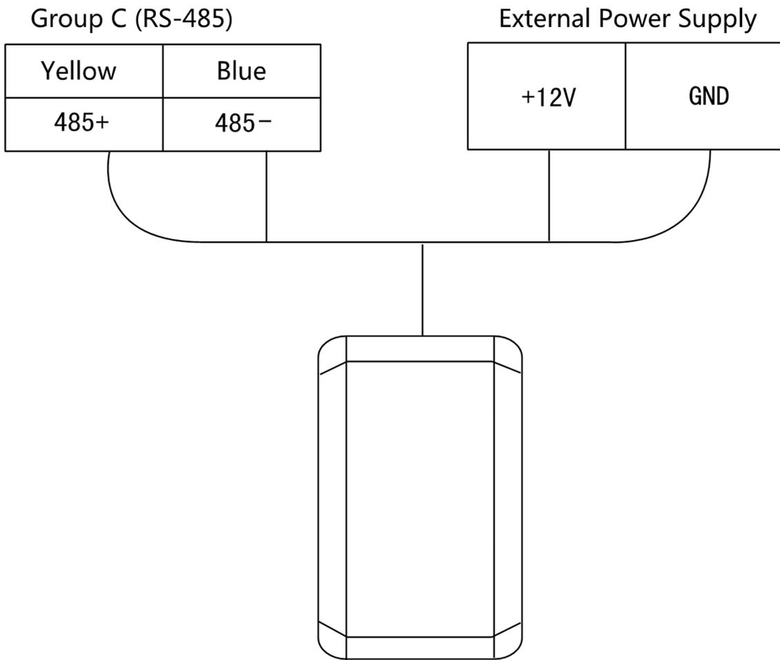
Figure 4-3 Wiring of External RS-485 Card Reader
