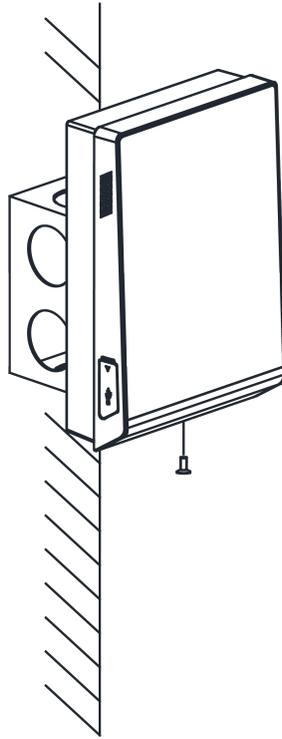
Figure 3-4 Tighten Screw
