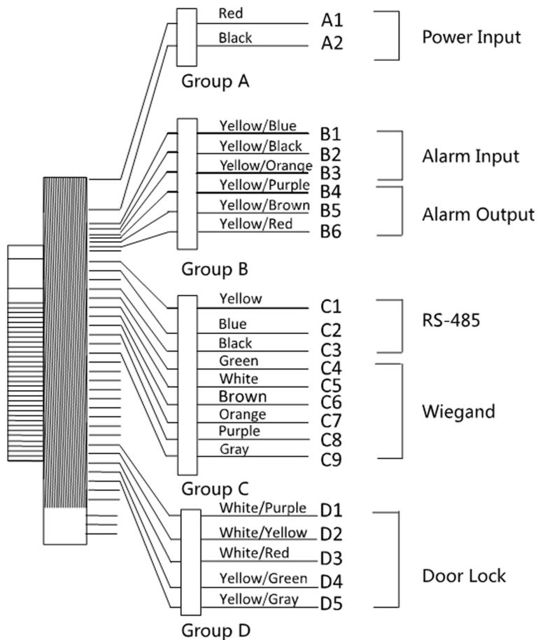
**Figure 4-1 Terminal Diagram**
